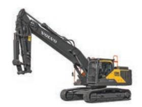
try-first feature called Lifting Volvo CE's new EC300E Straight Boom is a purpose-built demolition excavator with a max reach of more than 10 metres.
