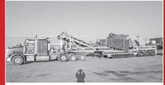
2020 UNIVERSAL 150/150/M2358/IMPACT CRUSHER with a 600Hp elect. Mtr and switchgear on a triple axle chassis. Like
