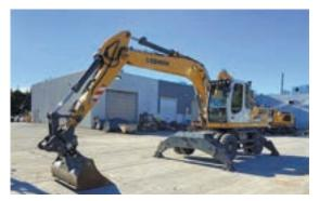
Liebherr A904C 2013 Material Handler, equipped with A/C, auxiliary hydraulics high pressure and medium pressure lines, automatic greaser, angled mono boom 5.30m, stick 2.65, lock valves boom and stick cylinders, rear camera, reversible fan, 4 outriggers, twin tires 10.00-20
