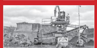
2742 CEDARAPIDS JAW CRUSHER self contained with a 17 foot vibratory feeder with a 3306 Cat Diesel Power unit, on a Triple axle chassis. Includes structure to mount a hammer or mini Ex on top and has a 42"Front discharge belt. Good Condition .......\$250,000 CAD
