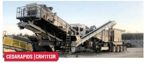
Closed circuit impactor/screen plan, 6'x16' 2-deck inclined screen, 450 HP T4F Scania diesel with hydraulic clutch crusher/generator drive, 150KW generator, 48" x 18' vibrating grizzly feeder with 6' stepped 2-deck grizzly, high production, high value plant.
