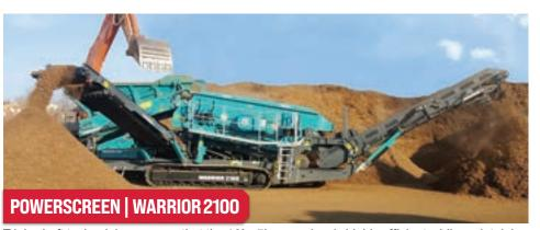
Triple shaft technololgy ensures that the 16' x 5' screen box is highly efficient while maintaining exceptional throughput productivity. The extreme screening acceleration offers the Warrior 2100 improved capabilities over its class rivals, especially in sticky scalping applications, screening and recycling applications. Features include a 16'x5' 2 deck screenbox, 9.2yd3 rigid one piece hopper, CAT C4.4 125hp.
