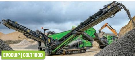
13'6" x 4' - 2 deck screen, variable screen angle, configurable layout/ability to convert to 2-way split, wide range of screen media, quick set-up time, reversable side conveyors, 55kW/74hp @2300rpm CAT engine.
