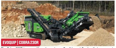
The Cobra 230R is a versatile and easy to use Small Impact Crusher that can operate in the most demanding of applications such as Reinforced Concrete, Recycled Asphalt, Construction and Demolition waste. Features include a 3.4yd3 hopper capacity, 34" crusher inlet, 8' x 4' single desk mesh screen, 281hp.
