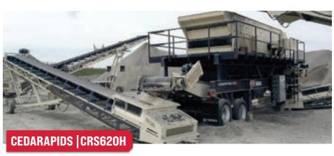
6' x 20' TSV6203 screen, flex shaft screen drive, rollaway blending chutes. Wide conveyor belts handle peak load conditions easily. Designed to get the most out of the screen so there is plenty of capacity to make the crushers the bottleneck in the circuit, not the screen.
