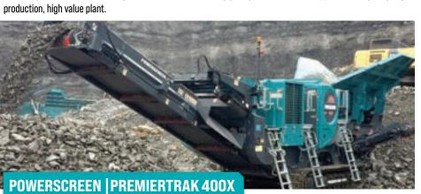
The Powerscreen® Premiertrak 400X range of portable jaw crushers are designed for customer operators in quarrying, demolition, recycling and mining applications. Hydraulic crusher setting adjustment for total control of product size and crusher overload protection to prevent damage by uncrushable objects.
