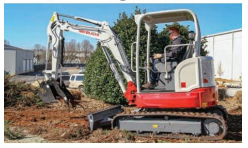
force of 4,290 lbs (19.1 kN). The excavator is powered by an EPA Tier 4/ EU Stage V delivering 24.4 hp (18.2 kW)
