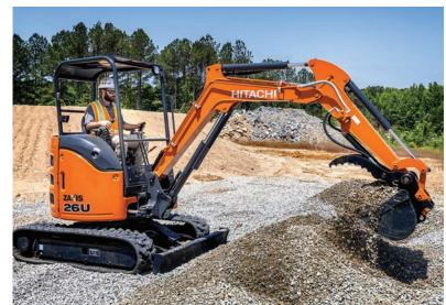
The power mode provides higher that allows the operator plenty of engine speeds for most general foot room. digging work, while the economy mode reduces engine speed for in lower noise and decreased fuel consumption.
