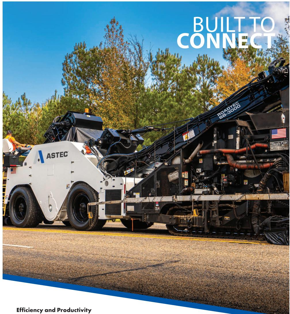
Designed with safety and operator comfort in mind, the Shuttle Buggy® material transfer vehicle features adaptive cruise control, bright LED lighting, four-wheel steering for easy transport and ground-level maintenance access for added convenience. Operators can rely on clear sightlines and the ground operator is safely protected inside the structure of the machine. The Roadtec SB-3000 is the perfect blend of traditional craftsmanship and modern technology.
