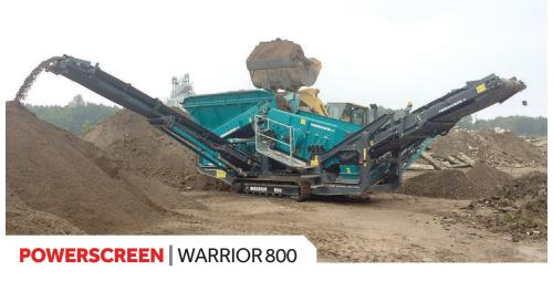
Multi-purpose heavy duty incline 2-deck 9'x4' screen,  $6.15 \text{ yd}^3$  variable speed hopper, rear wall collapsible for direct feeding, heavy duty variable speed belt feeder, hyd. folding conveyors. Capable of stockpiling, 3 way splitting or scalping before/after crushing units. Can accept bofor bars, finger screens, woven mesh and punch plate.
