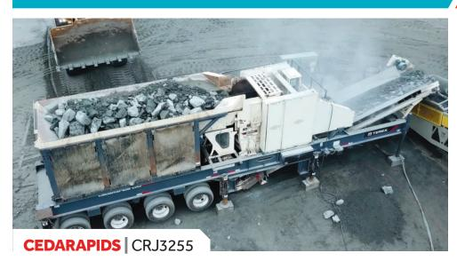
The Cedarapids CRJ3255 jaw plant combines the popular JW55 jaw crusher with the high stroke 52"x20' vibrating grizzly feeder making this plant a high production portable crushing machine. This quarry duty JW55 crusher, with its large 32"x55" opening, long jaws, and aggressive stroke, is in a class by itself in a portable crushing plant.
