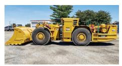
auto lube, spring applied hyd. release brakes, ejector bucket.
