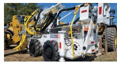
**Boart Stopemate** – Underground approved, hydraulic cylinders, fully pneumatic, ideal for captive areas and narrow vein mining.
