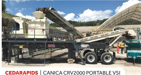
Features the Canica 2000 Vertical Shaft Impactor, available in a number of chamber configurations. Highly mobile all electric plant with the latest CCM automation system. Available in single or dual drive. Designed to handle a wide range of different applications and is well suited for manufacturing sand. Also available as a
