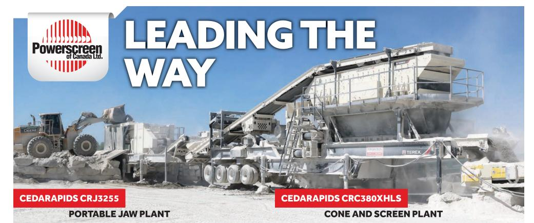
The Cedarapids CRJ3255 jaw plant combines the popular JW55 jaw crusher with the high stroke 52"x20' vibrating grizzly feeder making this plant a high production portable crushing machine. This quarry duty JW55 crusher, with its large 32"x55" opening, long jaws, and aggressive stroke, is in a class by itself in a portable crushing plant.
