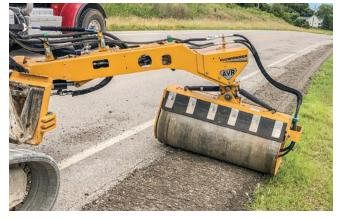
and are interchangeable. This allows road crews to take on jobs of varying sizes and aggregates by purchasing additional drums instead of investing in multiple self-propelled machines with engines that can fail. Additionally, the vibratory feature operates between 2,500-3,500 vibrations per minute for optimal compaction.
