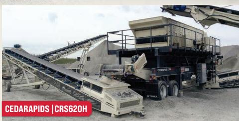
The Cedarapids® CRS620H screen plant features the popular  $6' \times 20'$  TSV6203 screen, along with a flex shaft screen drive and rollaway blending chutes, make this a leader in the screen plant market. The wide conveyor belts handle peak load conditions easily. Features include tool-less slope adjustment ( $0^{\circ}$  to  $7.5^{\circ}$ ), 48" underscreen conveyor, 30'' cross conveyors.
