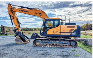
Cummins QSB6.7 engine with 182 hp, 51500 lb. op. weight, 18'8" boom, 9'7" arm, 2-way aux., piping w/ proportional joystick control, Hyundai hyd., QC., AMI hyd. thumb, Hyundai 42" bucket, pattern change selector valve, 32" triple grouser shoes, travel alarm, Hi-Mate remote management system, 620 hours ...
