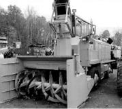
SMI 7200 ribbon blower, rebuilt 1997 G.M. V-12.
