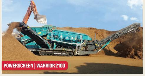
Triple shaft technololgy ensures that the 16' x 5' screen box is highly efficient while maintaining exceptional throughput productivity. The extreme screening acceleration offers the Warrior 2100 improved capabilities over its class rivals, especially in sticky scalping applications, screening and recycling applications. Features include a 16'x5' 2 deck screenbox, 9.2yd³ rigid one piece hopper, CAT C4.4 125hp.
