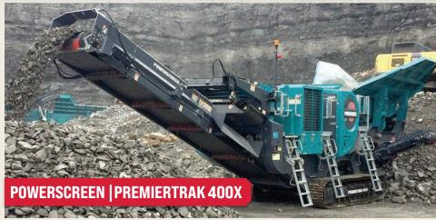
The Powerscreen® Premiertrak 400X range of portable jaw crushers are designed for customer operators in quarrying, demolition, recycling and mining applications. Hydraulic crusher setting adjustment for total control of product size and crusher overload protection to prevent damage by uncrushable objects.
