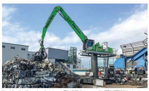
Material handler with a crawler undercarriage on a 15 foot (4.5 m) pylon powered by a 180 hp (132 kW) electric motor. This machine was purpose-built for the material handling conditions of Iwamoto Metal Co. Ltd.'s largest plant.
