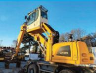
Liebherr LH24, Tier 4F, Cab elevation, Boom 6.10M, Stick 4.50M, Tool control
