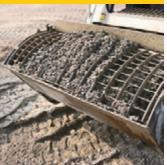
In takes just 3 minutes to mix components perfectly. Bucket capacity 100 to 2000 litres.
